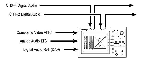
Figure 4: Connecting the standard 764 to your system
